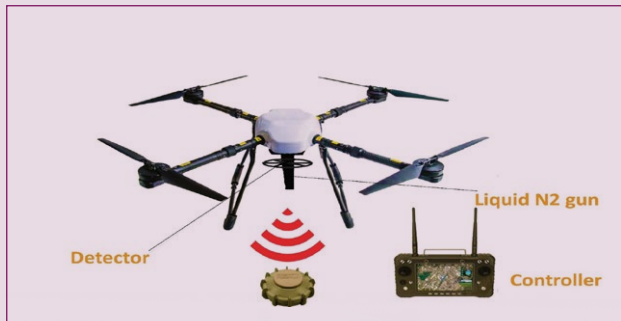
Figure 1: Method for detecting and securing mines using liquid nitrogen.
